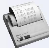
The output is sent to the printer each time the 3286-20 HOLD key is pressed.
