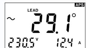
The 3286-20 provides the following 2 types of power factor measurement. If the waveform includes harmonic distortion, there will be a difference between the two measurement values, and the method must be selected accordingly.
