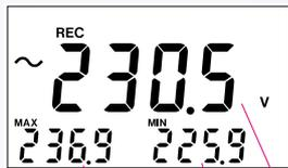
Using the record function, it is possible to check the amplitude of fluctuations.
