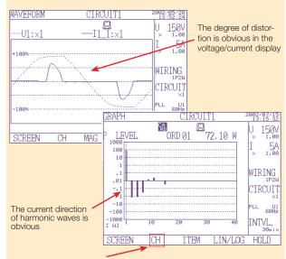
You can switch channels to easily check the harmonics for each circuit
