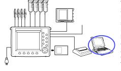
The 3169-20/21 includes an RS-232C interface as standard equipment. Using the RS-232C interface, settings of the 3169-20/21 can be made and measurement data can be acquired on a PC. This chapter explains how to connect the 3169-20/21 to a PC. For details including communications commands, see the RS-232C instruction manual (CD-R version).
