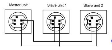
The slave units start time-series measurement, synchronized with the time-series measurement start signal output from the master unit.
