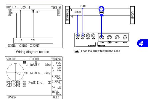
Wiring check screen (Power factor: 0.87) \$4.2.5 Checking the Wiring (page 49)
