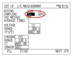
Press the **SET UP** key to display the setting screen.
