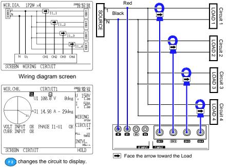
Wiring check screen (Power factor: 0.87) \$4.2.5 Checking the Wiring (page 49)
