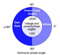
The arithmetic expressions for the harmonic-power phase angle vary depending on whether the reactive-power-meter method is ON or OFF.
