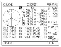
Wiring check screen (Power factor: 0.87)
