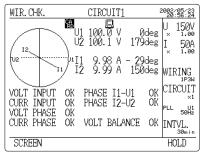
Wiring check screen (Power factor: 0.87)
