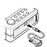
To connect the 3169-20/21 to a PC, you need the optional 9612 RS-232C cable. The 9612 RS-232C cable is a cross cable.
