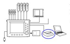
The instrument can produce hard copies of the screen and print measurement data on the Model 9442 PRINTER connected to the RS-232C interface.
