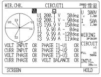
Wiring check screen (Power factor: 1)
