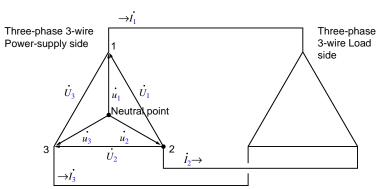
The figure above shows an artificial circuit of a three-phase 3-wire line. In the figure,  $\dot{U}_1$ ,  $\dot{U}_2$ , and  $\dot{U}_3$  represent the vectors of line to line voltage;  $\dot{I}_1$ ,  $\dot{I}_2$ , and  $\dot{I}_3$  represent the line (phase) current vectors;  $\dot{u}_1$ ,  $\dot{u}_2$ , and  $\dot{u}_3$  represent the phase to neutral voltage vectors. Normally, three-phase power P is obtained as the sum of the power of the phases.
