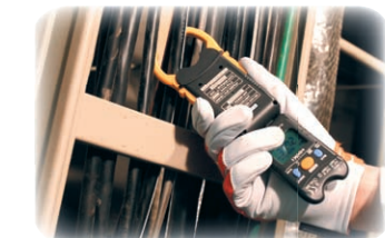
Sometimes it's easier to clamp the target wire at an angle.
