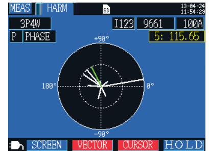
Harmonic power phase angle graph screen
