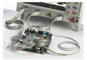
Designing with Altera or Xilinx FPGAs? Use the FPGA dynamic probe for rapid internal FPGA measurements. Using I<sup>2</sup>C, SPI, RS-232, or low- or full-speed USB? Use the digital channels to acquire and decode these buses, preserving analog channels for other timecorrelated measurements.
