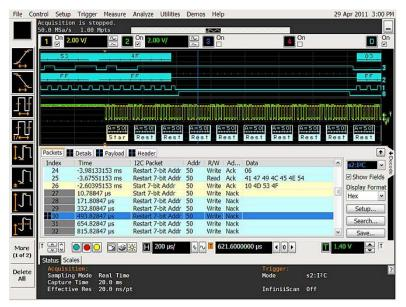
Use any combination of analog or digital channels for serial protocol decode, with up to four buses decoded simultaneously.
