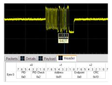
Header tab shows packets in a databook format. Hovering on any tab reveals additional detail.
