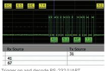
Trigger on and decode RS-232/UART transmission.
