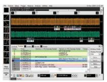
Trigger on and decode PCIe serial packets.
