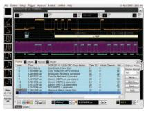
Trigger on and decode MIPI packets
