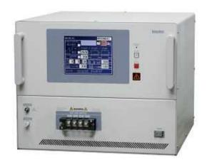
This Simulator unit is compliant with Damped Oscillatory Wave Immunity Test required by IEC60255-22-1 1 MHz burst immunity tests for measuring relays and protecting equipment. Also, it is capable to execute the other 100KHz Slow Damped Oscillatory Wave immunity test defined in IEC61000-4-18 2006 ed1.0.
