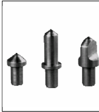
Short diamond indenter Slim diamond indenter Flat diamond indenter
